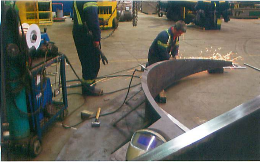
▲ The mild steel sculpture was plasma-cut, formed, rolled, and welded.
